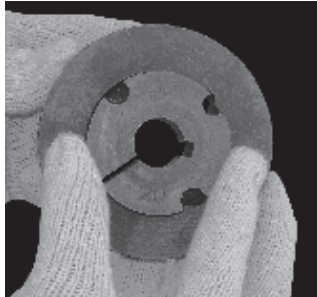
Step 1: First insert the bush in the pulley.
