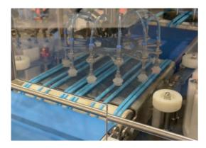
Megaweld thermoplastic polyurethane, trapezoidal and round belts are manufactured by a unique extrusion process. They are suitable for a wide range of applications and industries.
