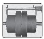
• Locate the coupling halves and element assembly approximately in the desired position. HRC couplings are required to be mounted with an allowance for a small amount of float. This internal float allows for any linear expansion and maintains the coupling's misalignment capability.
