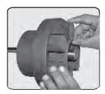
• To ensure correct mating of the two hubs, ensure that coupling-assembled, total length is correct.
